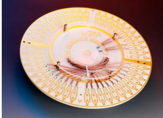
Figure 13. STAR's Parametric Test Probe Card
