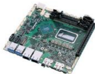
CPU Board SX-8030 Core™ embedded 6th Gen Skylake Up to 32GB
