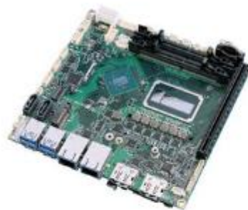
CPUボード SX-8030 Core™ 搭載 6th Gen Skylake Up to 32GB
